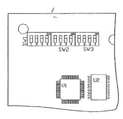
**SW1** dip-switch 2, 3, 4 set the maximum current of the charger. See table below for the dip-switches settings
